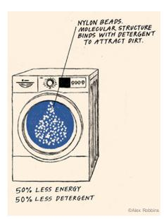
A British company called Xeros is transforming the automatic washing machine — an appliance that has changed little in 60 years — with technology that uses thousands of polymer beads to remove stains from clothes. The molecular structure of the beads combines with detergent to attract dirt. They can be used for hundreds of washes before being recycled.
