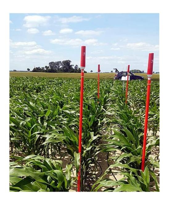
In 2004, PlantCare developed a novel Soil Moisture Sensor that combines a number of key advantages over all other known sensor types. Therefore, the sensor based on a micro-thermal measurement has already established itself in all sectors, as can be seen from the approximately 250,000 pieces of sensors sold worldwide.
