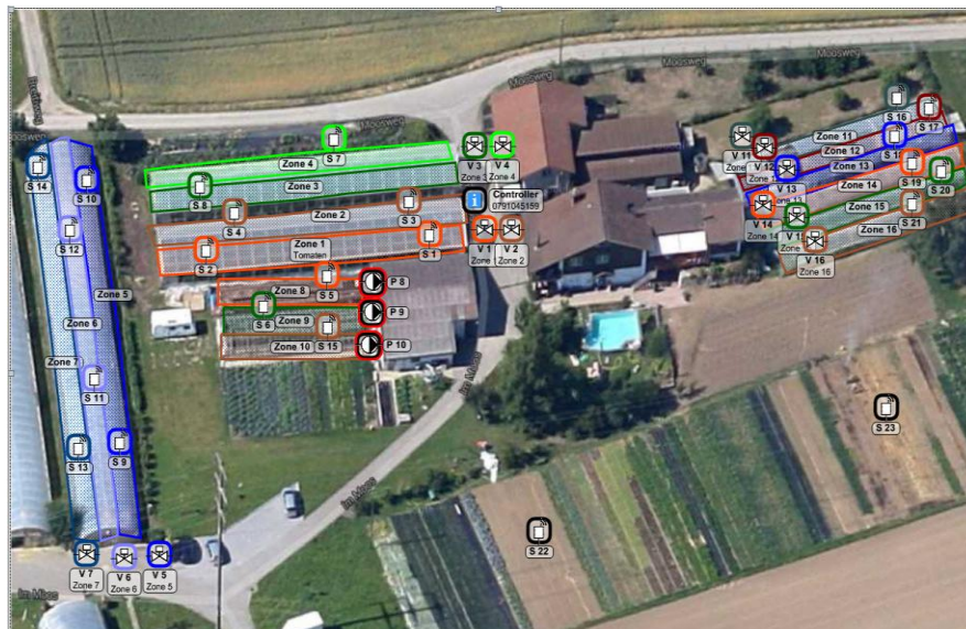
Fig. 11: This smallholder farm contains 16 irrigation zones of which 4 are irrigated using the semi-automatic mode, 8 use the fully-automatic mode and 4 are cloned zones.
