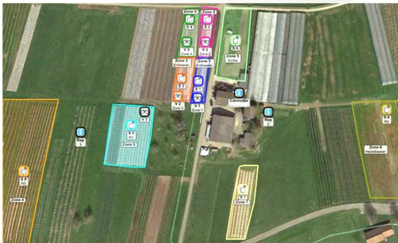
Fig.2: Arrangement of the irrigated areas, the sensors , valves and radio repeaters
