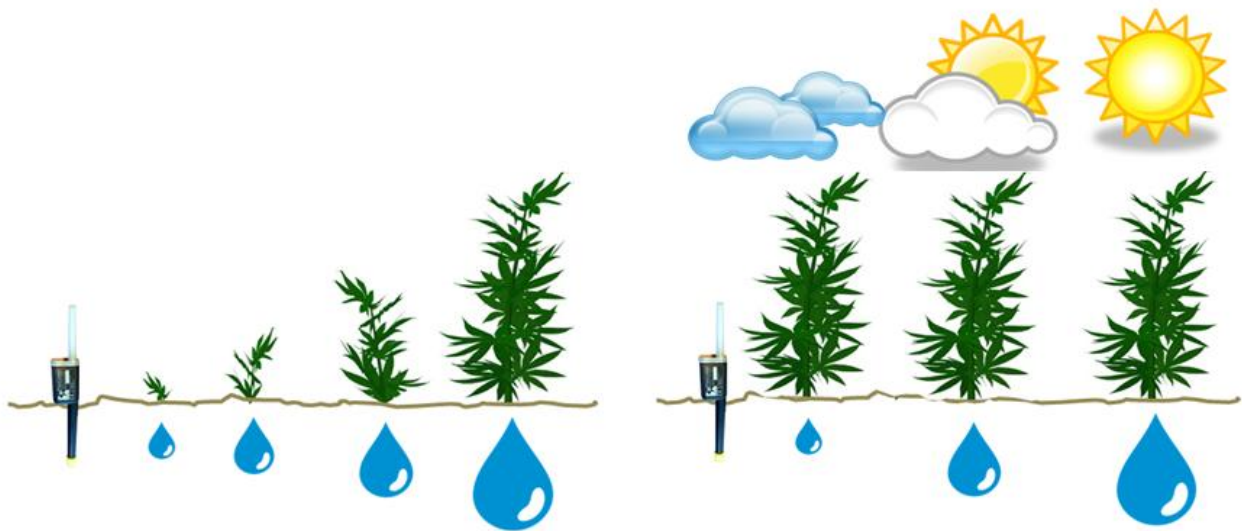
Fig.15. The DRA method eliminates any manual readjustment of the irrigation duration.
